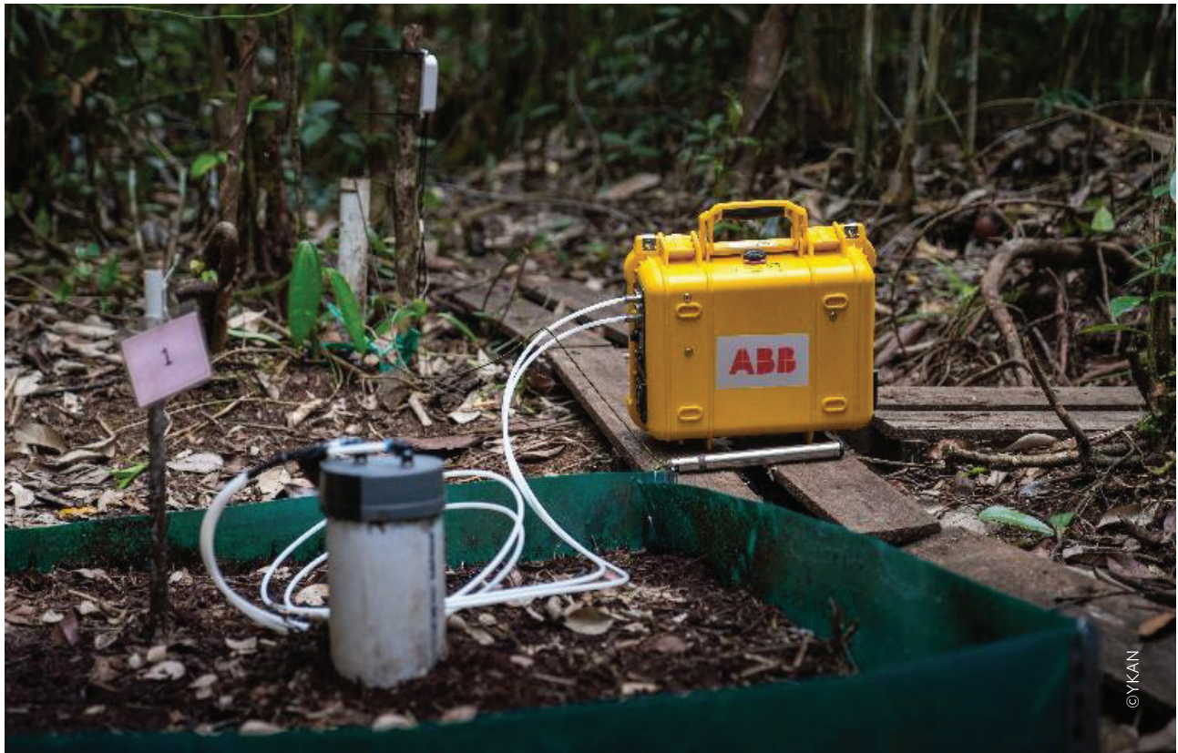
Figure 4. LGR-ICOS™ GLA131 Series with a developed close chamber system
